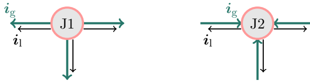
(b) Relation between the global axis, i_g , and the local axis, i_l , used by the network model.
