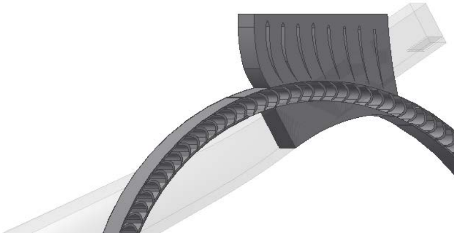
Figure 2. Novel partial admission compressor configuration
