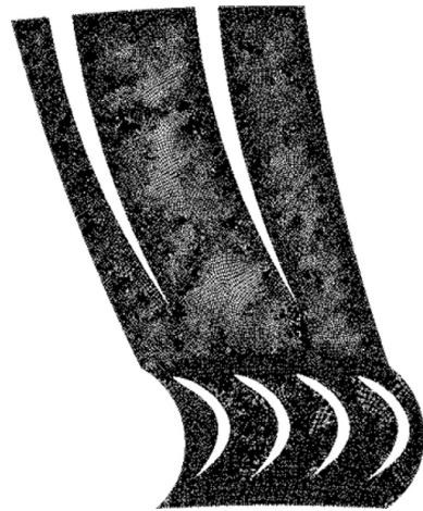
Fig. 14 – The meshed domain of 1/50 of the full wheel depicting the reference blade shape.
