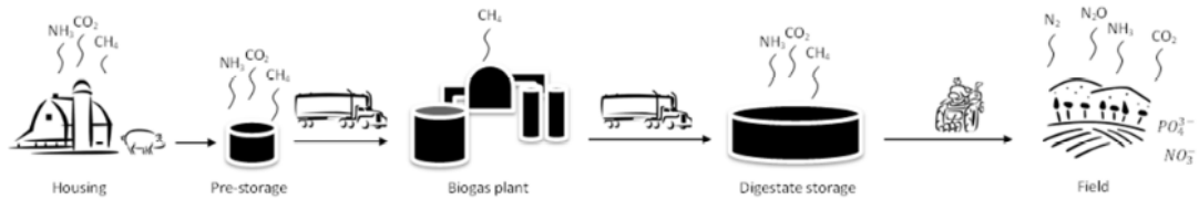
Figure 13. Manure management with biogas production (Vega, 2012)
