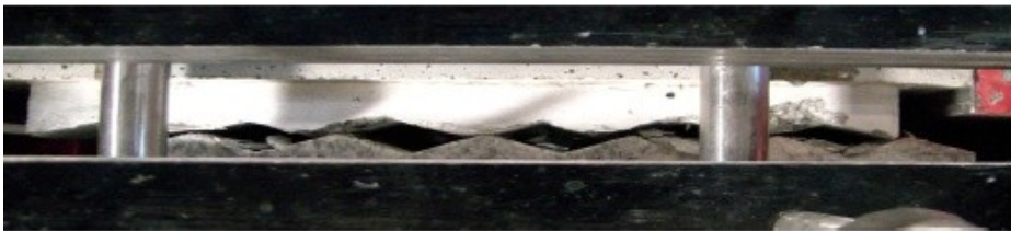
Test 2.1 after maximum displacement. Approximately 25mm
