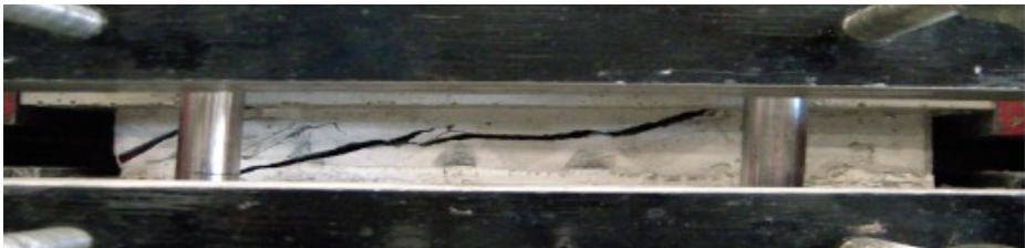
Test 1.3H after maximum displacement. Approximately 15mm
