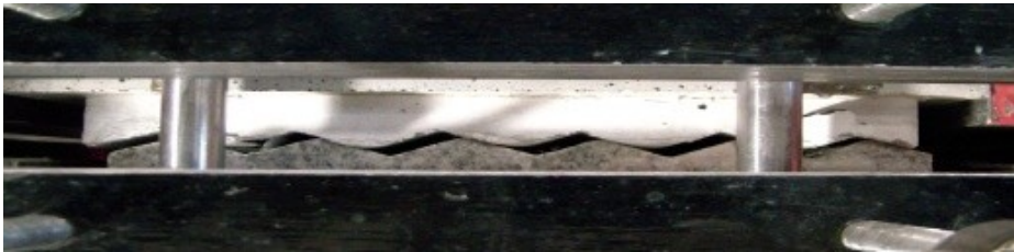
Test 2.1 at maximum capacity after approximately 6.4mm of displacement
