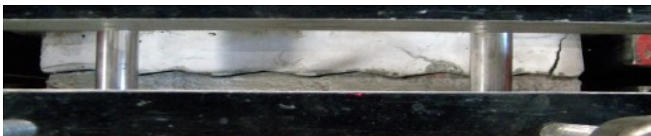
Test 3.3 at maximum capacity after approximately 2.8mm of displacement
