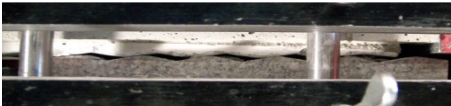
Test 3.1 after maximum displacement. Approximately 33mm
