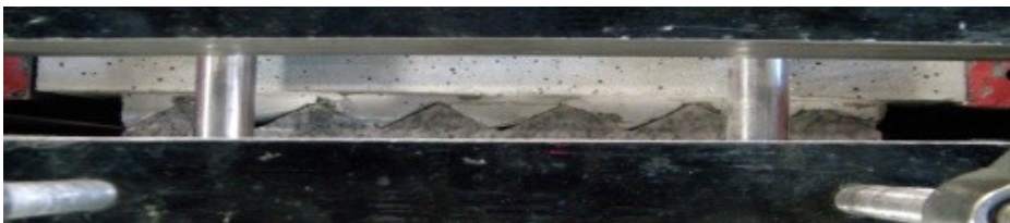
Test 1.4 at maximum capacity after approximately 1.4mm of displacement
