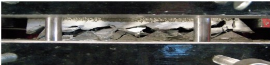
Test 1.1 after maximum displacement. Approximately 15mm
