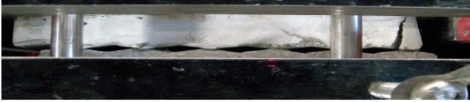
Test 3.3 after maximum displacement. Approximately 33mm
