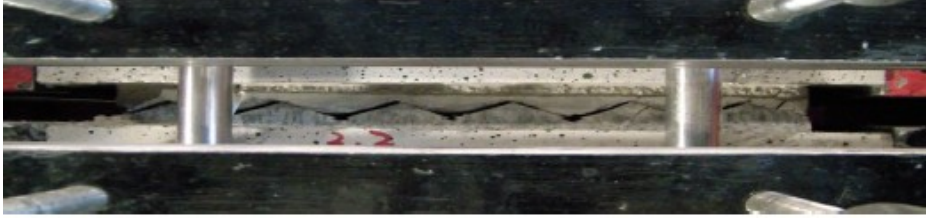
Test 2.2 at maximum capacity after approximately 2.9mm of displacement
