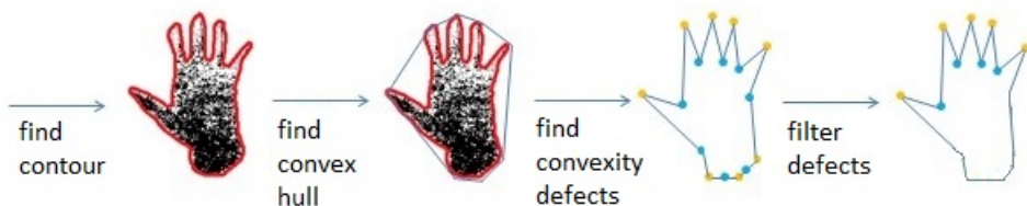
Figure 3.3: The process of finding the correct convexity defects after acquiring the binary image of the hand.
