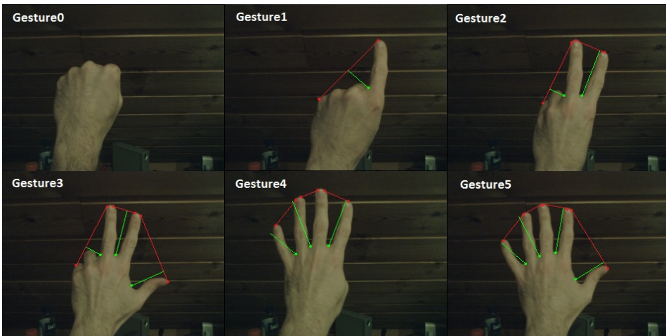
Figure 3.4: Examples of the 6 different gestures to be recognized with convexity defects drawn on. The red points represent the start- and end-points of the defects, while the green represent the point farthest away from the convex hull. The green line is the distance between the convexity defect and the convex hull and is orthogonal to the red line.
