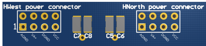
Figure 4.6: Mecobo power connectors
