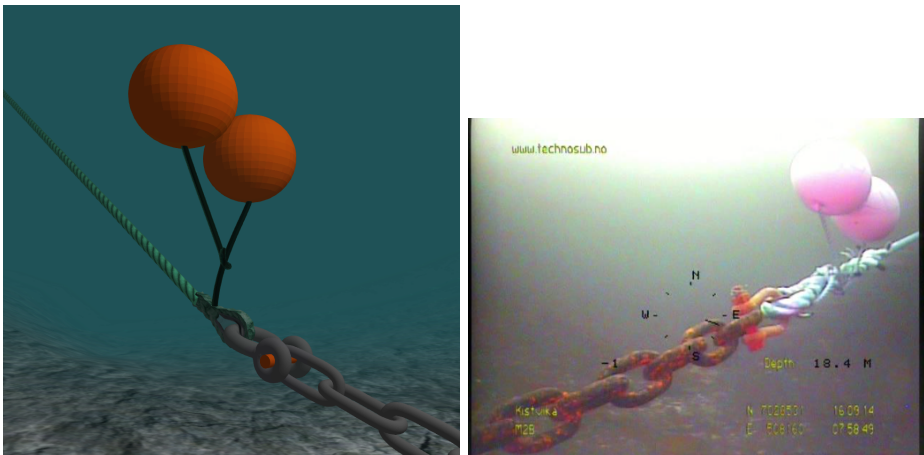
Figure 4.21: Comparison of the transition between rope and chain with an underwater buoy
