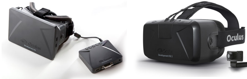
Figure 3.4: Oculus rift: DK1 (left) and DK2 (right)
