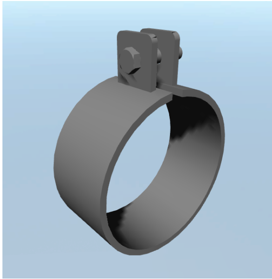
Figure 4.6: A bottom clamp that will be attached to a sinker ring
