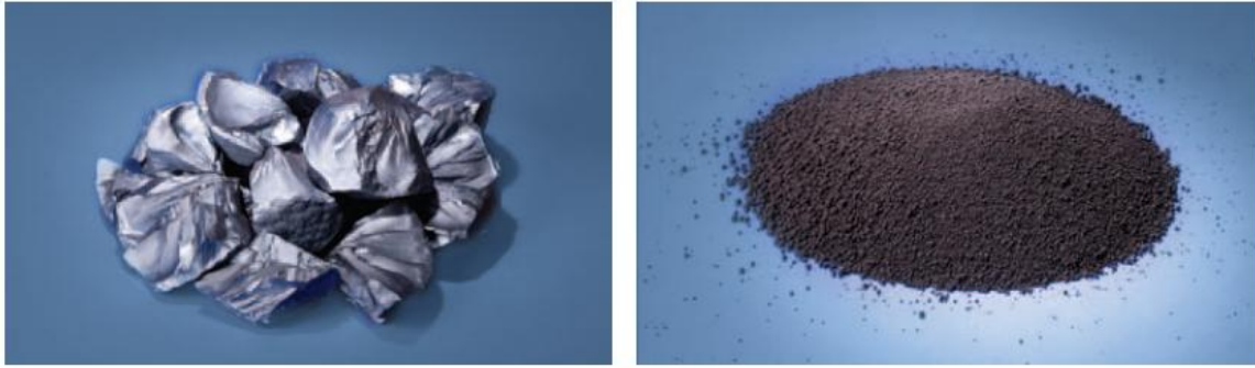
Figure 6.5: SoG-Si in form of Siemens chunks (left) and FBR granules (right) (REC, 2011b).
