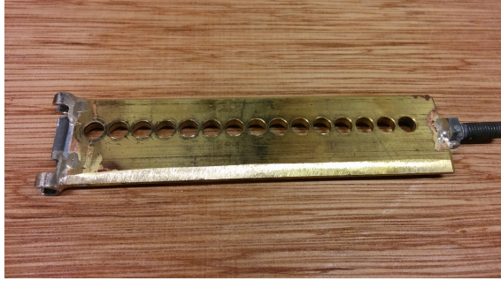
Figure 2.15: the manual traverse device used to move the 5-hole Pitot in horizontal direction.
