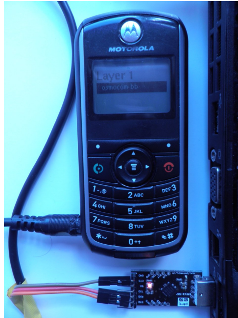
Figure A.1: Motorola C118 connected to a computer with a CP2102 USB to serial converter.
