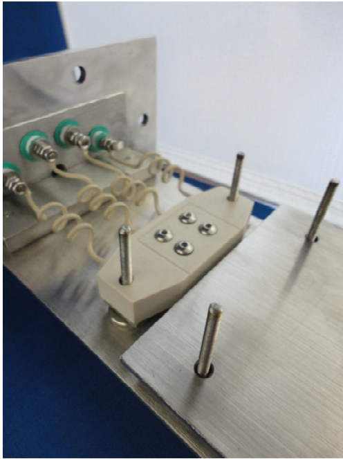
Figure 2a. TPS PEEK High Temperature Adaptor positioned on sample / sensor insert
