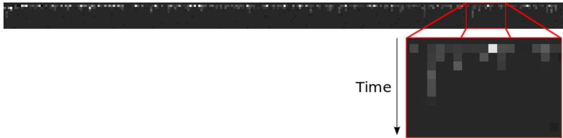
Figure 4.1: The figure show part of a raw timing measurement on the target platform. The bleeding of cache misses into subsequent measurements is clearly visible in the excerpt. More white denote longer access time.
