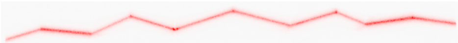
Figure 3.8: An laser image taken of the calibration object as seen when calibrating the top camera. The image has been inverted to avoid the black background.
