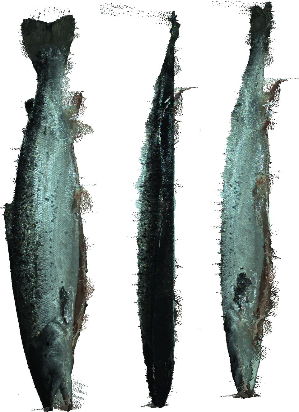
Figure 3.13: An image of Fish16 in the data set, obtained without a polarization filter. Increased noise is present around fins and sharp edges due to reflections of laser light. Left: Side view, Middle: back view, Right: tilted abdominal view
