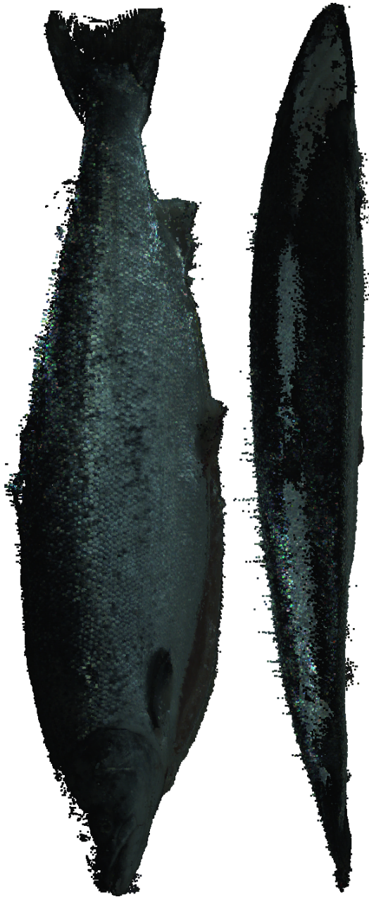
Figure 3.12: A scan obtained of a salmon using a polarization filter. The lighter areas on the back indicate missing coordinates (the points from the bottom are seen through the gaps).
