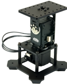
Figur 4.2: WidowX MX-28 Pan Tilt Kit fra Trossen Robotics.
