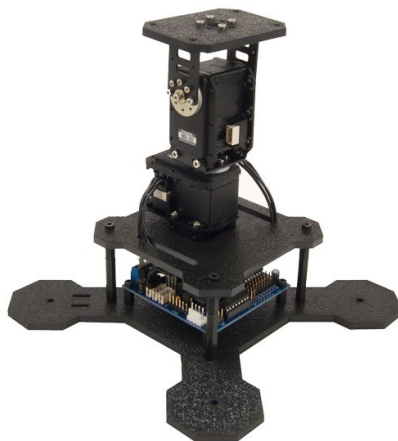
Figur 4.3: WidowX MX-28 Robot Turret Kit fra Trossen Robotics.
