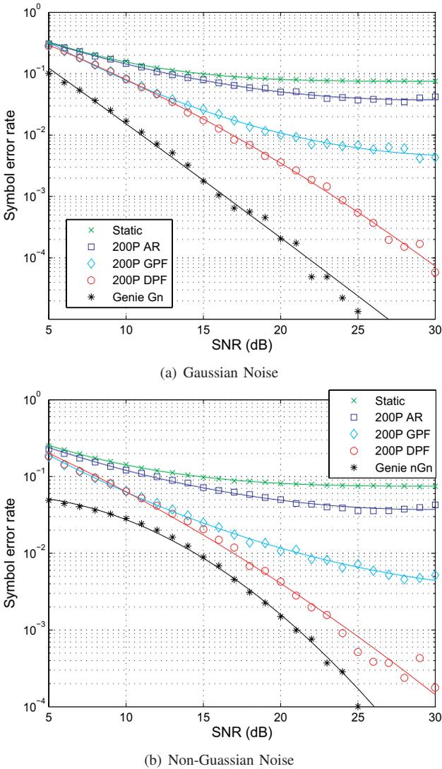
Fig. 4. Symbol error rate vs. SNR for the different receiver types for both Gaussian (a), and non-Gaussian noise. In the highly dispersive channel the particle filter using the dynamic AR model provides the best results.
