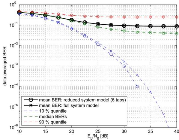
Fig. 1. Comparison of reduced equivalent system model performance with full system model performance; determined (averaged) over 1000 different equivalent system models.
