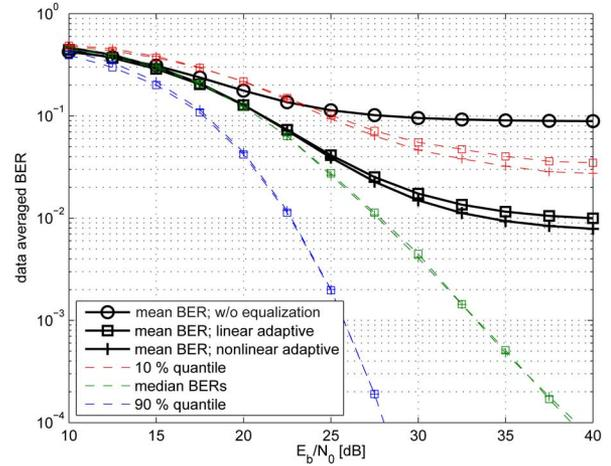
Fig. 3. Comparison of adaptive equalizers with 50 000 training symbols and an exponentially decreasing step size; Performance evaluated by analyzing over 800 equivalent system models.
