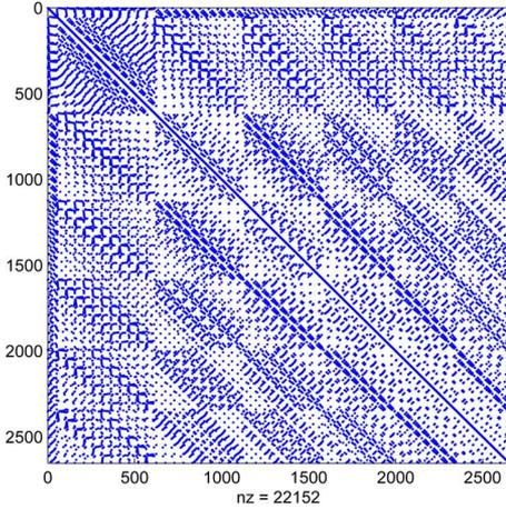
Fig. 5. Autocorrelation matrix of the data vector  $\mathbf{r}[k]$ . The matrix has  $2652 \times 2652$  elements, where 22 152 are nonzero which reduces computational complexity because of the sparsity.
