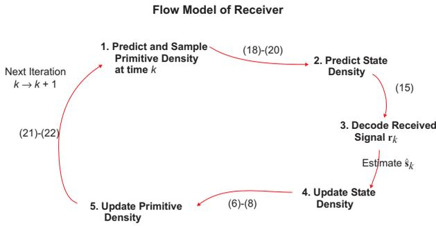
Fig. 3. Flow-graph illustrating how to incorporate a dynamical AR module. The goal is to model the changes in the channel as a Gaussian distribution whose mean and variance correspond to the parameters of the parametric AR(1) model given by (21) and (22).
