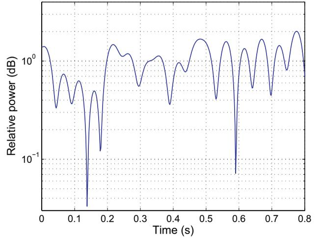
Fig. 2. A typical Doppler faded channel realization. For this fading rate ( $f_D T_s = 0.01$ ) there are two deep fades at times 0.14s and 0.6s respectively. During these instances the static AR model of (10) is ill-suited for providing predictive channel estimates.
