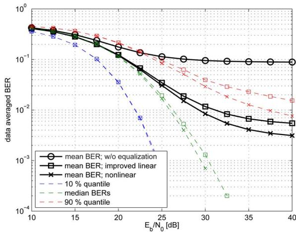
Fig. 2. Comparison of derived MMSE equalizers; linear and second-order equalizer performance analyzed over 800 different equivalent system models.
