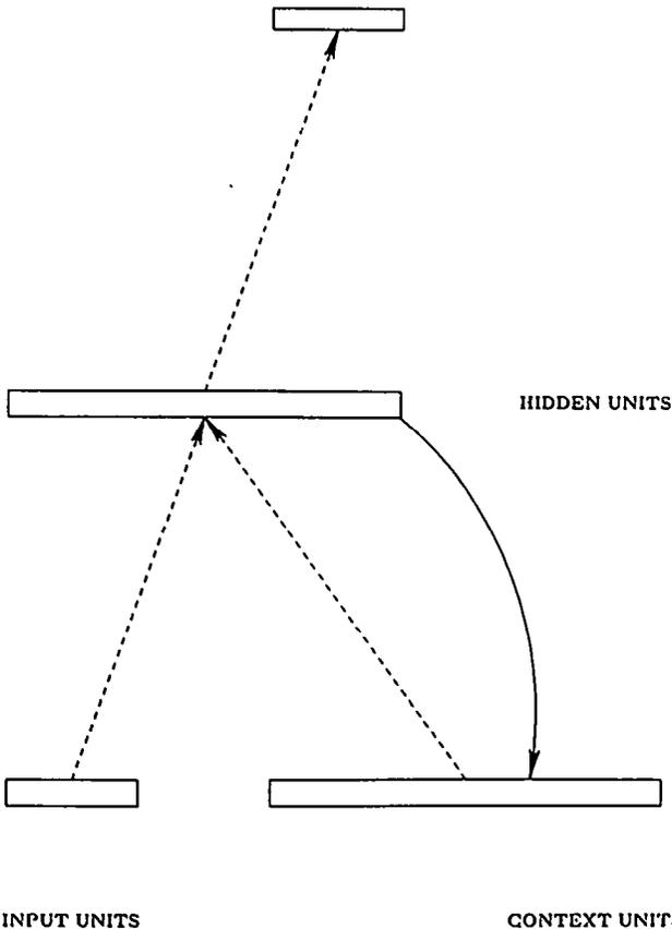
**Figure 2.** A simple recurrent network in which activations are copied from hidden layer to context layer on a one-for-one basis, with fixed weight of 1.0. Dotted lines represent trainable connections.
