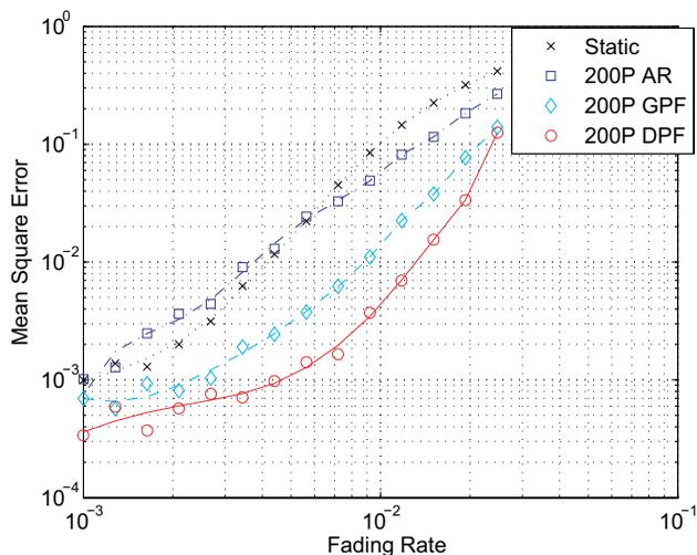
Fig. 6. Mean squared error tracking performance (averaged over all channels) vs. normalized Doppler rate.
