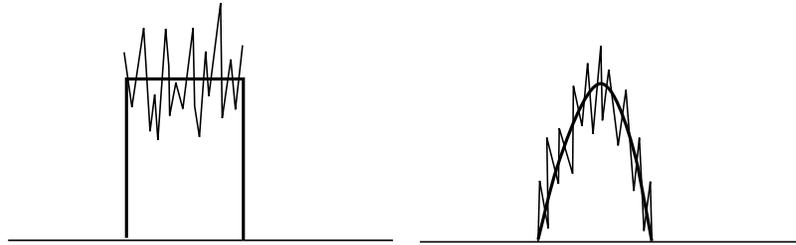
**Fig. 10 – The effect of noise on the average signal to noise ratio is different for these two pulses.**
