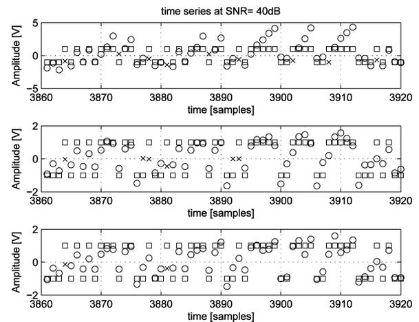
Fig. 4. Time series of distorted data symbols (top), data symbols after the linear equalizer (middle), and data symbols after nonlinear equalizer (bottom). “□” denotes the originally transmitted symbol, “o” denotes correctly detected symbol for each equalizer, and “x” denotes incorrectly detected data symbol for each equalizer, respectively.
