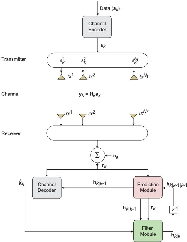
Fig. 1. Block receiver design structure incorporating the channel tracking modules.
