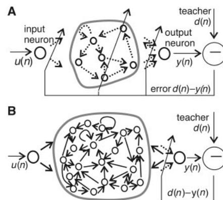
**Fig. 1.** (A) Schema of previous approaches to RNN learning. (B) Schema of ESN approach. Solid bold arrows, fixed synaptic connections; dotted arrows, adjustable connections. Both approaches aim at minimizing the error  $d(n) - y(n)$ , where  $y(n)$  is the network output and  $d(n)$  is the teacher time series observed from the target system.
