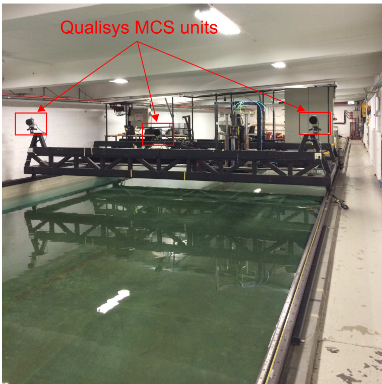
Figure B.7: MCLab model basin. Three Qualisys MCS units marked with red boxes.
