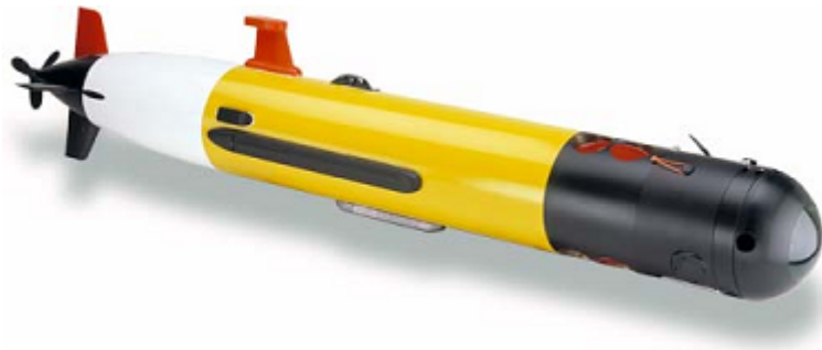
Figure 1.2: Kongsberg Maritimes AUV Remus 100, from http://www.ntnu.edu/amos/aur-lab
