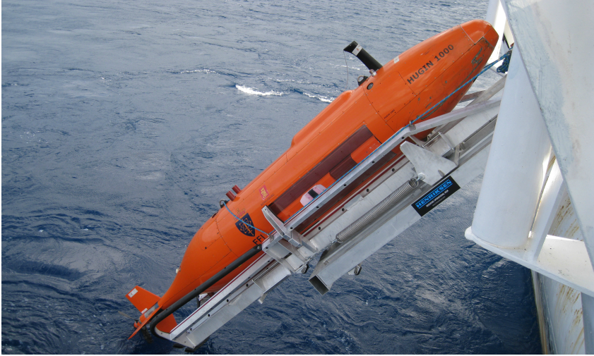
Figure 2.1: The HUGIN 1000 AUV
