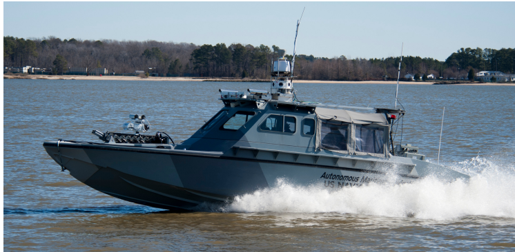
Figure 2.5: Powervent USV prototype, the second of three USV prototypes used in the AMN project (image courtesy of U.S. Navy).
