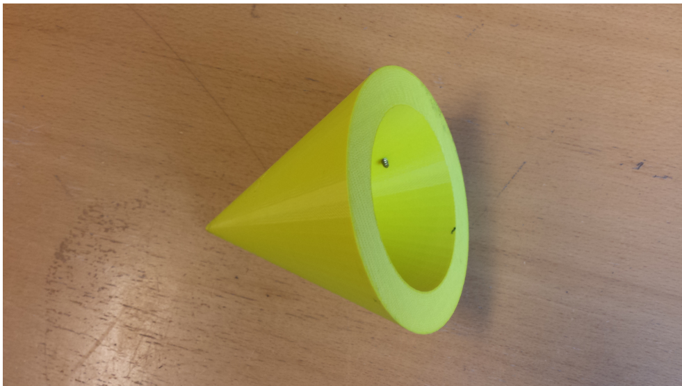
Figure 3.4: Test beacon with the milled-out back visible
