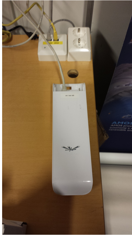
Figure 6.2: Nanostation M connected to the internal network on the ground station
