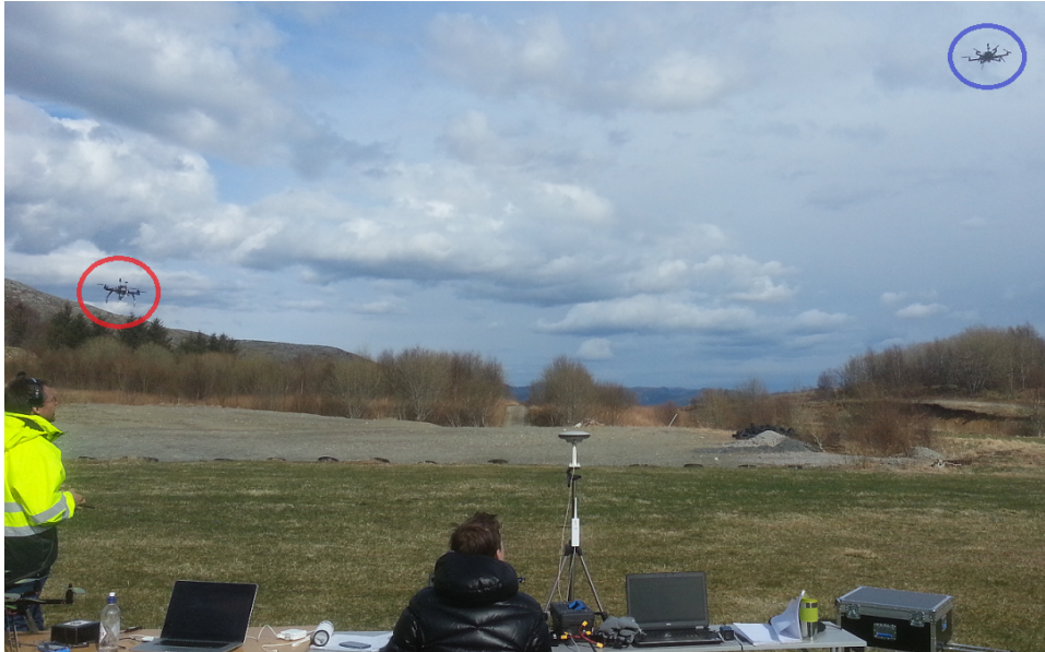
Figure 7.4: Photo of Rover 1 and 2 at the start of Experiment 1-3, marked by their respective colors of blue and red. One of the pilots is also present, as well as the base station and the GCS with operator.
