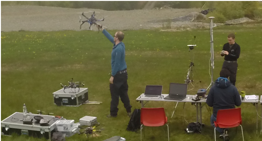
Figure 7.2: The experimental setup at Agdenes Airfield. Co-supervisor Kristian Klausen can be seen performing a magnetometer calibration on one of the multirotors, while the author inspects the base station antenna. Collaborative MSc student Recep Cetin is seen manning the GCS next to the base station.
