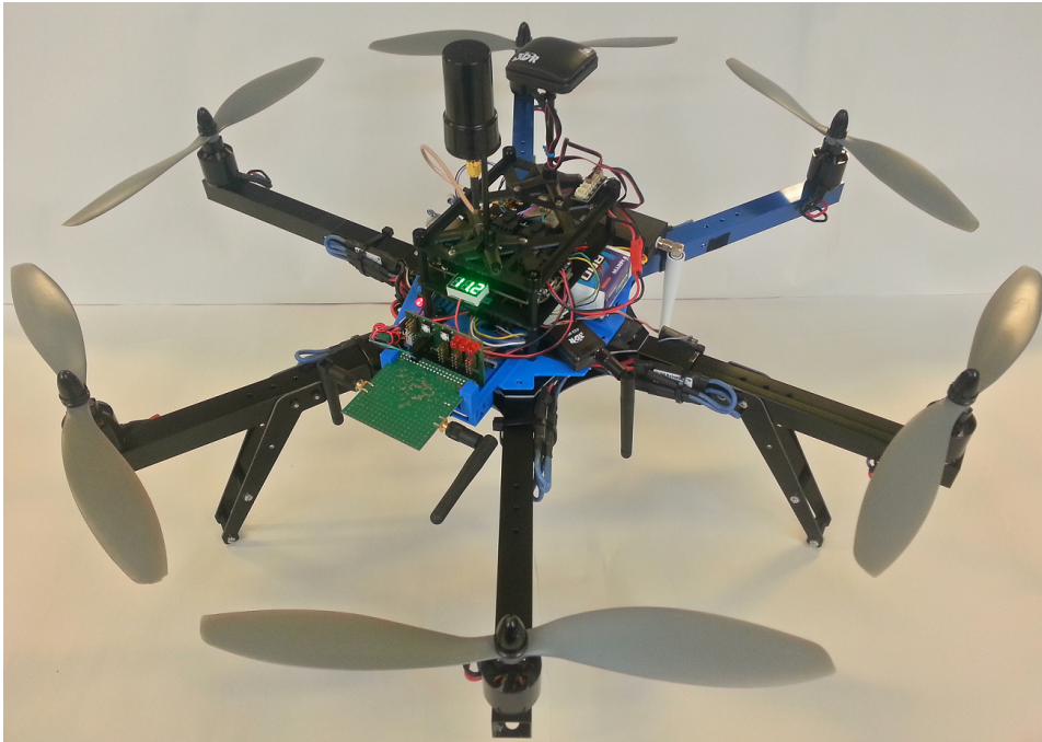
Figure 2.1: The complete multirotor with the custom payload and all components.
