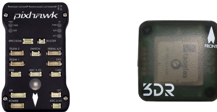
(a) The Pixhawk autopilot. Image courtesy of 3drobotics.com. (b) The GPS/compass module. Image courtesy of 3drobotics.com.
