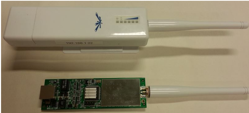
Figure 2.9: The PicoStation M2 HP from Ubiquiti Networks, with and without its plastic housing.
