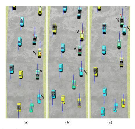
**Figure G.3:** A variation of the harsh braking incident from experiment 7 with symmetric road traffic.  $v_k$  is braking to avoid a blue vehicle in front (Figure G.3a) and  $v_i$  is braking to avoid  $v_k$  (Figure G.3b), the braking is too harsh and  $v_i$  suffers a rear-end collision from  $v_j$  (Figure G.3c).
