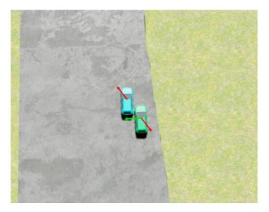
**Figure D.1:** The blue vehicle in front is trying to avoid the green vehicle entering the road from the right. Because of the vehicles driving 10% slower of what they are allowed to do, the blue vehicle can increase its speed to allow the green vehicle entrance on the road without colliding.
