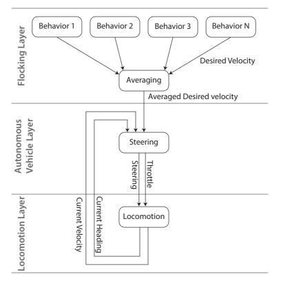
**Figure 3.1:** An overview of the layered model that controls a vehicle. The Desired Velocity and the Averaged Desired Velocity are vectors.
