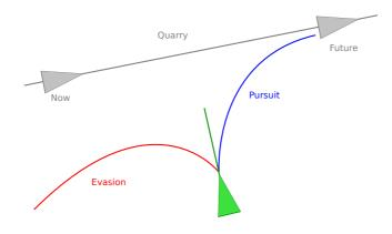
**Figure 2.4:** This figure shows the overall idea of the pursue and evasion steering behavior. The key is to predict the future position of a quarry (target). (Adopted from: Reynolds [1999])
