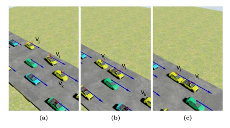
Figure 5.2: An incident from Experiment 2, with throughput above 9000. Occasionally our PID controller can brake more harshly than intended and cause incidents.
