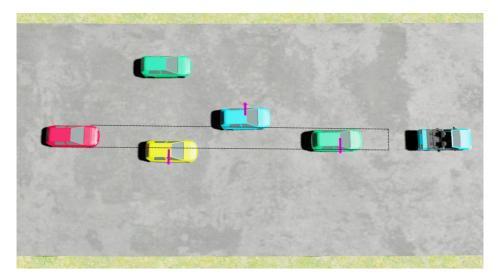
Figure 3.17: An emergency vehicle with its reserved area in front. The emergency vehicle have no constraints on where in the road to drive and ordinary vehicles in front will move to the closest side to escape the reserved area. The AP Behavior is illustrated as purple arrows.
