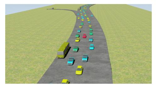
**Figure 4.5:** A typical road traffic scenario when both buses, emergency vehicles, merging traffic, and oncoming traffic is active. Note the areas in front of the emergency vehicle and the buses that are cleared due to the AP Behavior.
