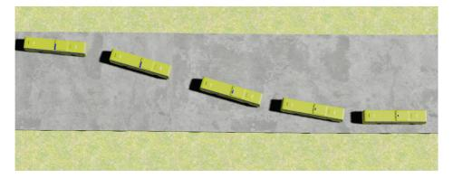
Figure 3.18: The Keep Right Behavior (KR) is non-linear and produces a steering vector with a larger magnitude if the bus is on the left-hand side than if the bus is on the right-hand side.
