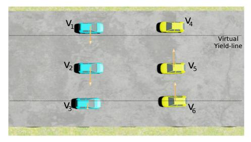
**Figure 3.15:** An illustration of three important attributes of the Avoid Oncoming Behavior (AO). See the text for details. AO is the behavior aimed at ensuring oncoming vehicles do not collide. The virtual yield-line is only drawn for illustrative purposes and is not drawn in the actual simulations.
