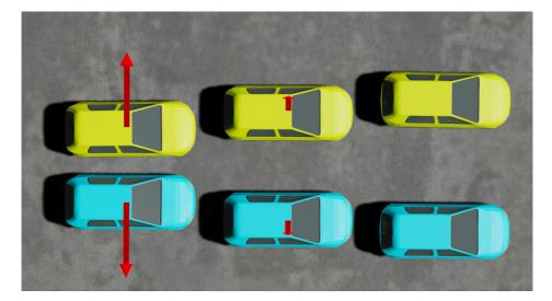
**Figure 3.9:** The Avoid Behavior urges vehicles to keep a minimum distance between themselves. If two vehicles come too close, the Avoid Behavior will generate a steering vector that points directly away from the other vehicle. The generated steering behavior is here illustrated as a red arrow starting from the vehicle center and pointing away from the other vehicle.
