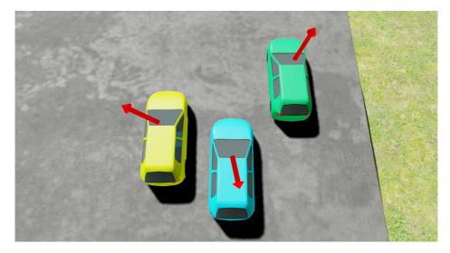
**Figure 3.10:** A vehicle could have multiple other vehicles that are too close. An avoidance vector will be computed for each vehicle that are too close and summed up to form the final avoidance steering vector.
