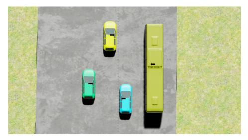
**Figure 3.21:** The Cohesion Behavior can be thought of a creating a virtual line between the center of a group of vehicles that the group will try to align themselves on laterally.
