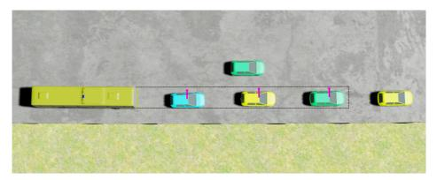
**Figure 3.16:** Avoid Prioritized (AP) works by reserving an area in front of the vehicles with higher priority. The area is illustrated by a dotted line in front of the bus. Vehicles in front of the high-priority vehicle will have to move out of the area to give way to the bus. The AP Behavior is illustrated as purple arrows.
