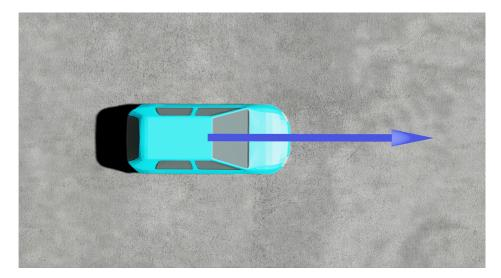
**Figure 3.8:** This figure illustrates the steering vector generated from the Road Tangent Behavior. This behavior urges the vehicle to follow the road. The steering vector is here displayed as a blue arrow pointing forward from the center of the car. The direction of the arrow indicates the desired driving direction, and the length indicates the desired speed.
