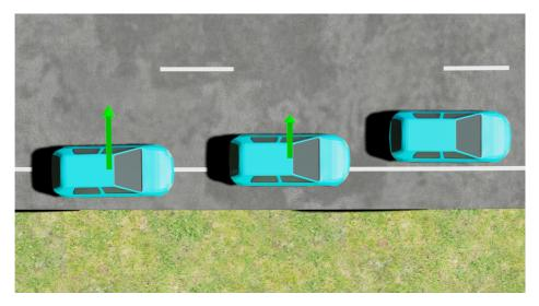
**Figure 3.11:** The KIR Behavior ensures that a vehicle remains on the road. The behavior is dynamical in the sense that it increases in strength as a vehicle approaches the edge of the road. In this figure, the green arrow illustrates the KIR Behavior as it urges the blue vehicles to steer to the left to avoid the edge of the road. We can see that the green arrow decreases in magnitude as the vehicle increases its distance to the edge.
