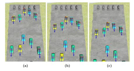
**Figure 5.1:** An illustration of how an incident due to the unstable spawning problem appears. The green vehicle in the top left is spawned next to a yellow vehicle that causes it to steer to its left. However, another yellow vehicle has already been spawned to the left, and the green vehicle does not have time to react. See the text for more detail.
