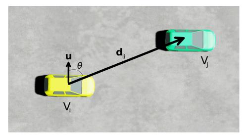
**Figure 3.20:** This figure illustrates the vectors and angles needed for computing the steering vector for the Cohesion Behavior. **u** is a unit vector that points to the side of  $v_i$ , and  $\mathbf{d}_{ij}$  is a vector from the center of  $v_i$  to the center of  $v_j$ .
