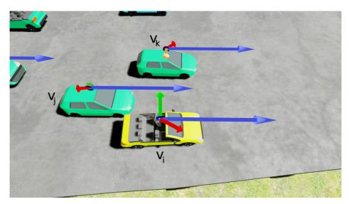
**Figure 5.7:** An example of an alignment incident that occurred in Experiment 7.  $v_k$  wants to steer right to avoid an oncoming vehicle,  $v_j$  is being squeezed in the middle and wants to brake, and  $v_i$  is merging and wants to steer left to enter the road. The result for  $v_i$  is that the lateral force of the KIR Behavior (green arrow) is stronger than the lateral force of the Avoid Behavior and  $v_i$  drives into  $v_j$ .
