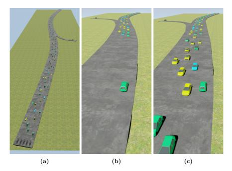
**Figure 4.2:** Scenarios describing Experiment 2. Figure 4.2a shows the five vehicle spawners located at one end, Figure 4.2b shows a single vehicle coming from the other end at the start of the experiment, and Figure 4.2c shows how asymmetric traffic looks in the simulation.
