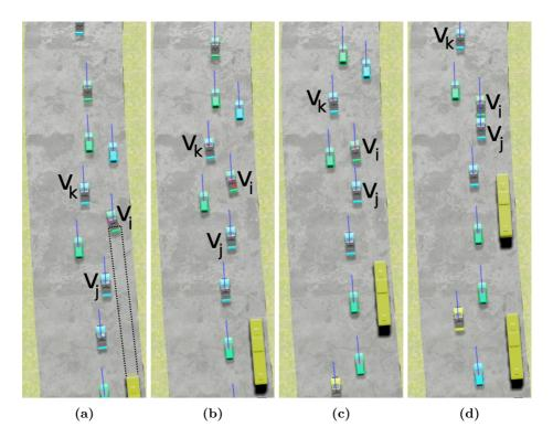
**Figure G.1:** Vehicle  $v_i$  ends up colliding with  $v_j$  due to harsh braking.  $v_i$  initially steers left to yield to a bus(Figure G.1a), then starts to brake to avoid  $v_k$  (Figure G.1b), then tries to accelerate again (Figure G.1c) but is too slow and an incident occurs (Figure G.1d).
