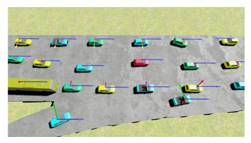
**Figure 3.7:** Multiple vehicles with their steering behaviors indicated by colored arrows. The final behavior of a vehicle will be a sum of the individual steering behaviors.
