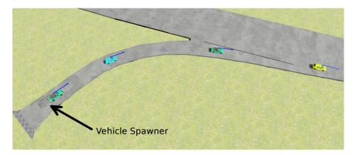
**Figure 3.19:** An illustration of vehicles on the entrance ramp entering the road. The vehicle spawner is located at the start of the ramp, and the dotted line is the virtual boundary for where the entrance ramp becomes road.
