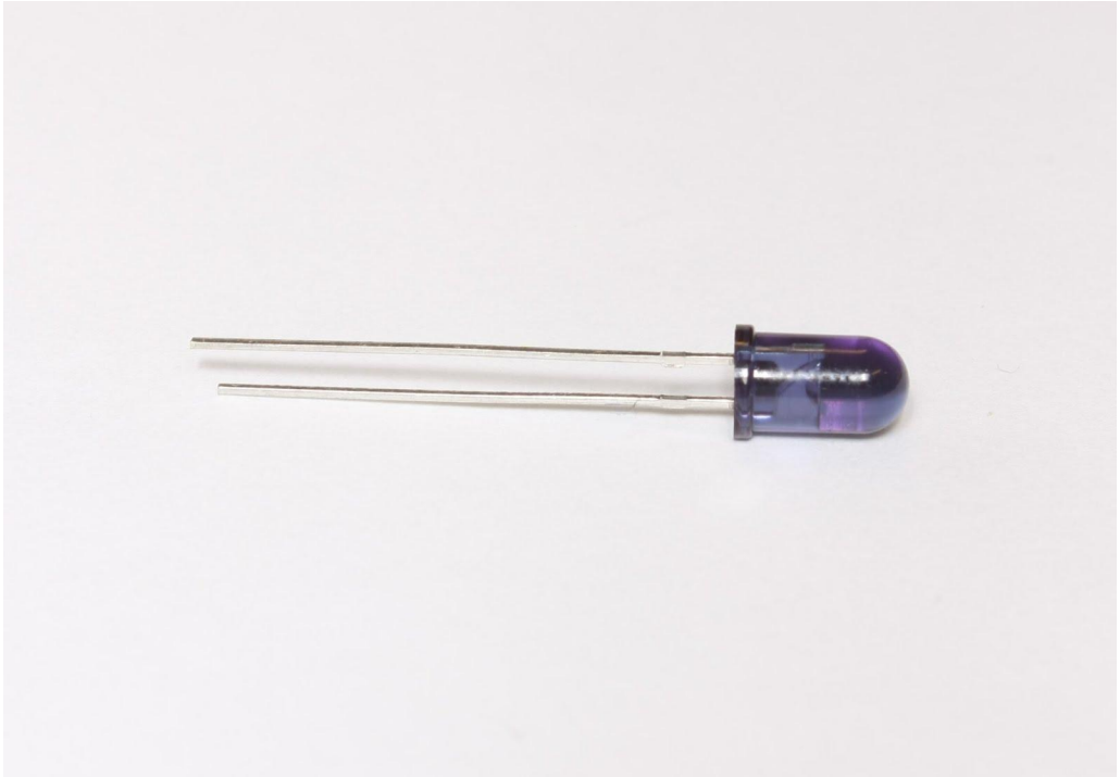
IMG12 Infrared Emitter LED the long leg is positive, and the short leg is negative.
