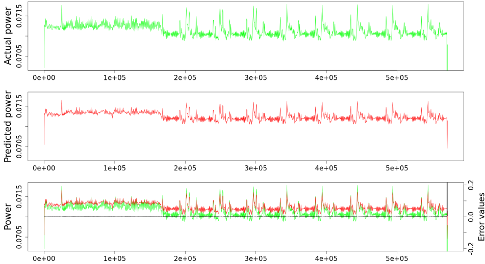
Figure 6.2: The predicted power consumption versus the actual power consumption versus the error per cycle of the validation benchmark. Power values are on the left axis, while error values are on the right.
