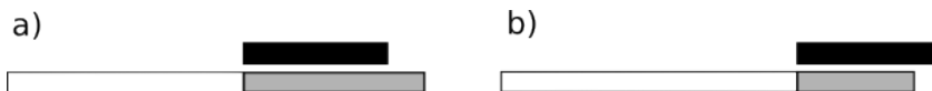
Figure 2.9: The two possible 3' adapter alignments. The black rectangle represents the adapter and its alignment to the read, and the grey rectangle shows the removed suffix.
