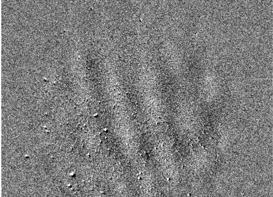
Figure 3: Difference image: the subtraction of two images of the OH airglow taken with an all-sky imager at Dragvoll, NTNU, Trondheim, November 18, 2012, at about 01:16.
