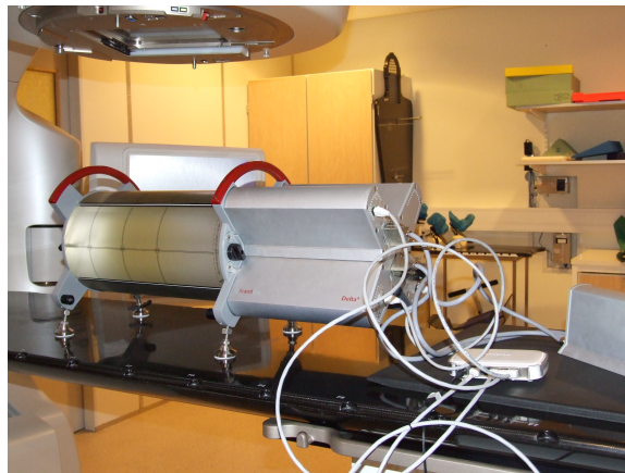
Figure 3.13: The Delta4 phantom used for verification of patient VMAT plans. The cylinder section to the left contains the detector arrays, the grey X-shape to the right contains the on-board electrometer and data processing units for relating charge to absorbed dose.
