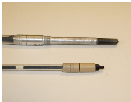
Figure 3.10: Top: Farmer ionization chamber FC65-G. Bottom: CC01 ionization chamber.
