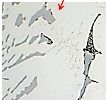
Fig. 3.34 – Optical micrographs at 100x magnification: AA 2618 (a), Zr-modified AA 2618 (b), Zr- and V-modified AA 2618 (c), enlargement of areas in the red rectangles, which show a fine phase dispersed in the matrix (d) and (e). In Figure 3.20 (a) the different types of phases detected are indicated: lamellar eutectic structure (1), needle-like black phase (2), light grey phase (3) and dark grey feather-like, lath-like or irregular phases(4). OP-S polished and not-etched samples.
