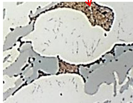
Fig. 3.34 – Optical micrographs at 100x magnification: AA 2618 (a), Zr-modified AA 2618 (b), Zr- and V-modified AA 2618 (c), enlargement of areas in the red rectangles, which show a fine phase dispersed in the matrix (d) and (e). In Figure 3.20 (a) the different types of phases detected are indicated: lamellar eutectic structure (1), needle-like black phase (2), light grey phase (3) and dark grey feather-like, lath-like or irregular phases(4). OP-S polished and not-etched samples.
