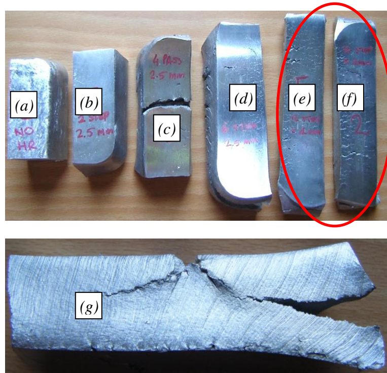
Fig. 3.30 – Hot rolled samples of Zr-modified AA 2618: as-cast sample (a), 16% (b), 33% (c), 50% (d), (e), (f) deformed samples, and enlargement of a 50% deformed sample (g). As explained in paragraph 2.2.5, samples (e) and (f), highlighted by the red circle, were hot rolled using different parameters from the other samples.
