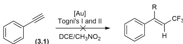
**Figure 4.2:** Illustration of the failed attempts at [Au]-catalyzed trifluoromethylation of phenylacetylene (**3.1**)
