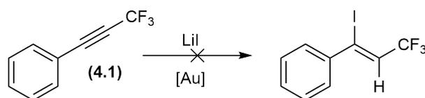
**Figure 3.10:** The attempted reaction to produce a trifluoromethylated vinyliodide.
