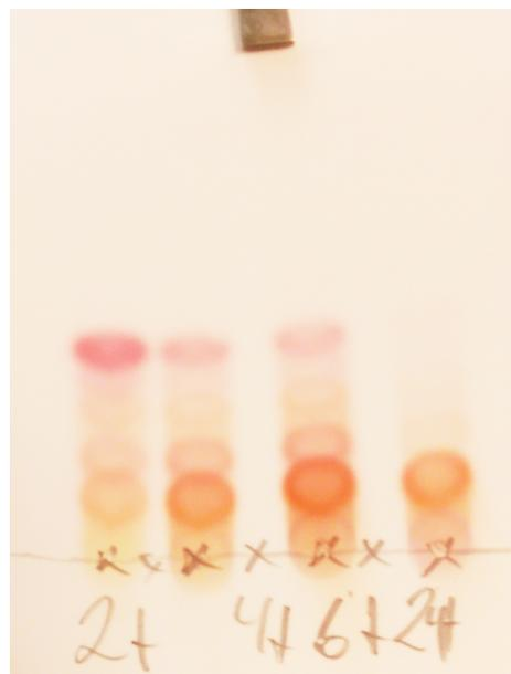
**Figure 3.1:** Picture of TLC-plate from reaction shown in Fig. 3.2. (Eluent: 10 % EtOAc in n-pentane)
