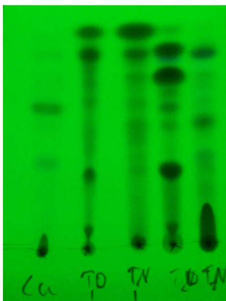
**Figure 3.4:** Picture of TLC-plate from reactions with [Au] and Togni's I and II. From left to right: Reference CuI reaction, Togni I and DCE, Togni I and  $\text{MeNO}_2$ , Togni II and DCE, Togni II and  $\text{MeNO}_2$ . (Eluent: 10 % EtOAc in n-pentane).
