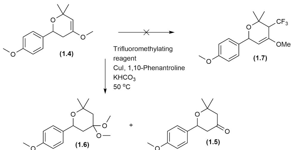
**Figure 3.2:** The attempted reaction of trifluoromethylation of (**1.4**). Tongi's I, II and Umemoto was tried in different reactions.
