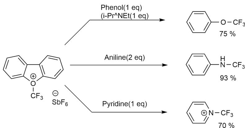
**Figure 2.12:** Some examples showing the possibilities with the oxygen variant of Umemoto's reagent.
