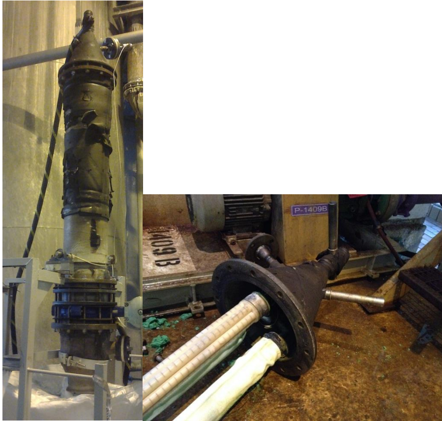
Figure 4.4: The left image shows the candle filter vessel. The right image shows of the demounted candles taken out of the container. The top candle is without a filter cloth while the bottom two candles are covered by a filter cloth.
