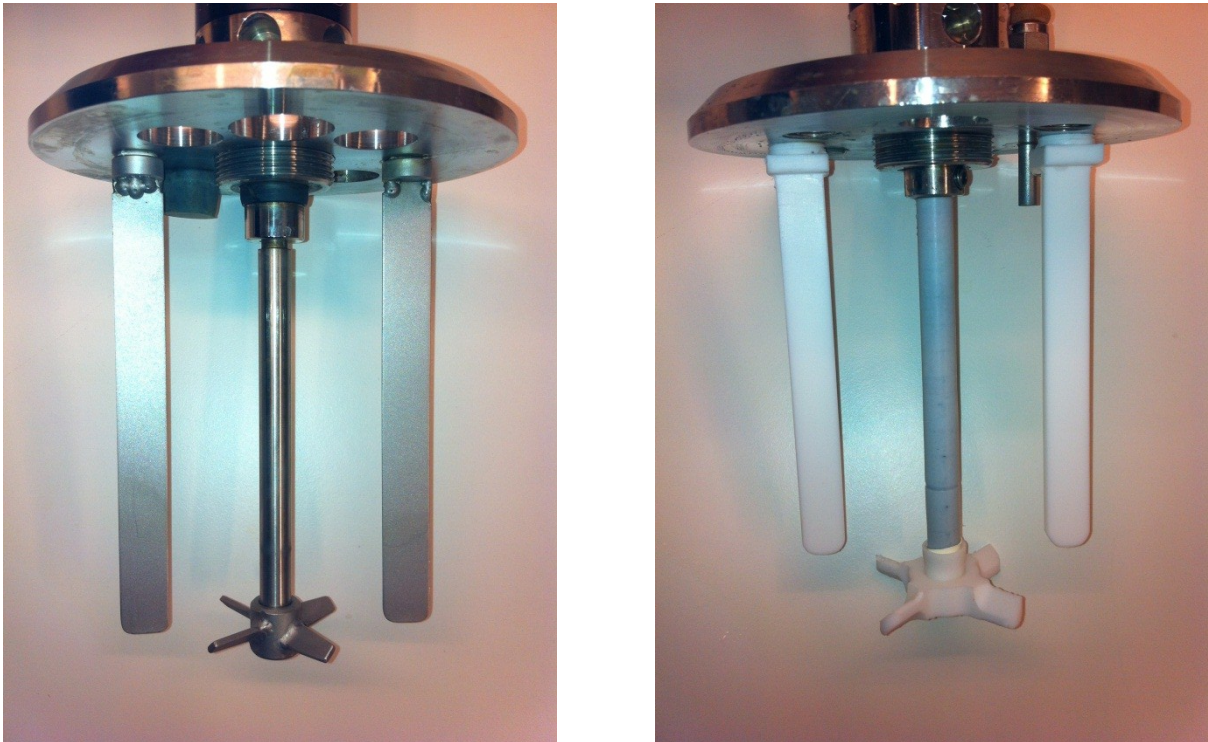
Figure H. 1: Reactor lid with propeller and baffles made of steel (left) and Teflon (right).
