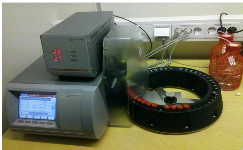
Figure 3.2 Density meter (Anton Paar DMA 4500M)
