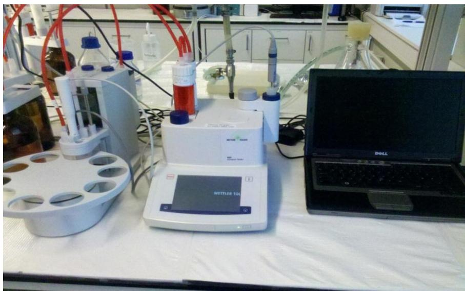
Figure 3.1(a) Mettler Toledo G-20 setup for amine analysis
