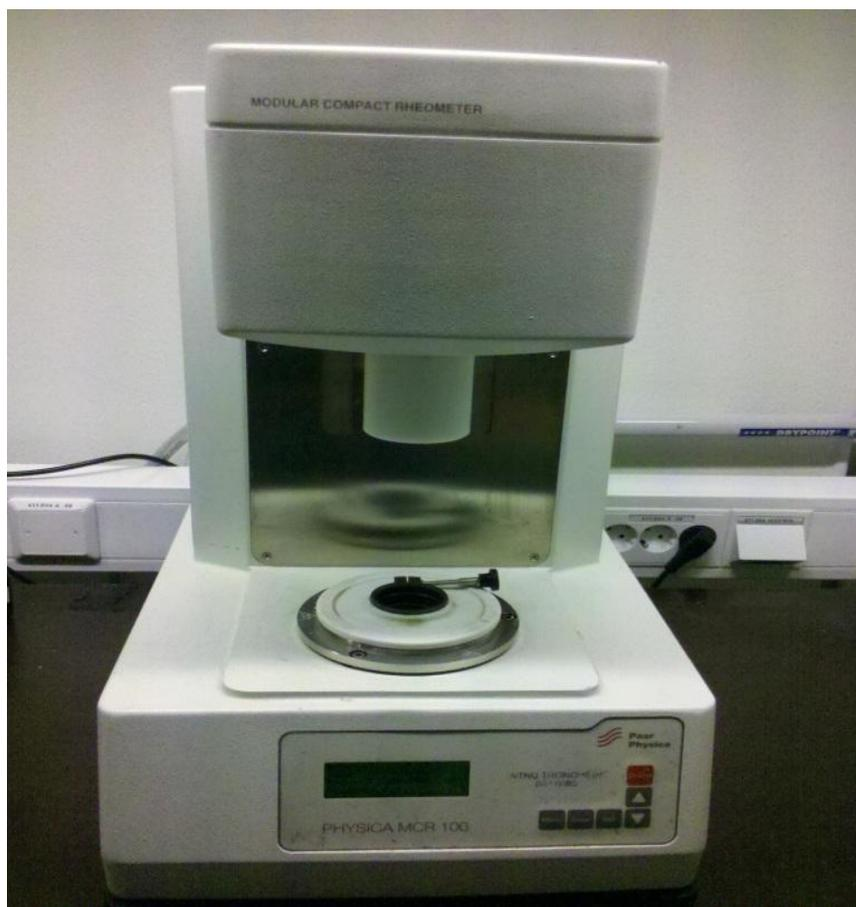
Figure 3.3 Physica MCR 100 rheometer setup for viscosity measurements
