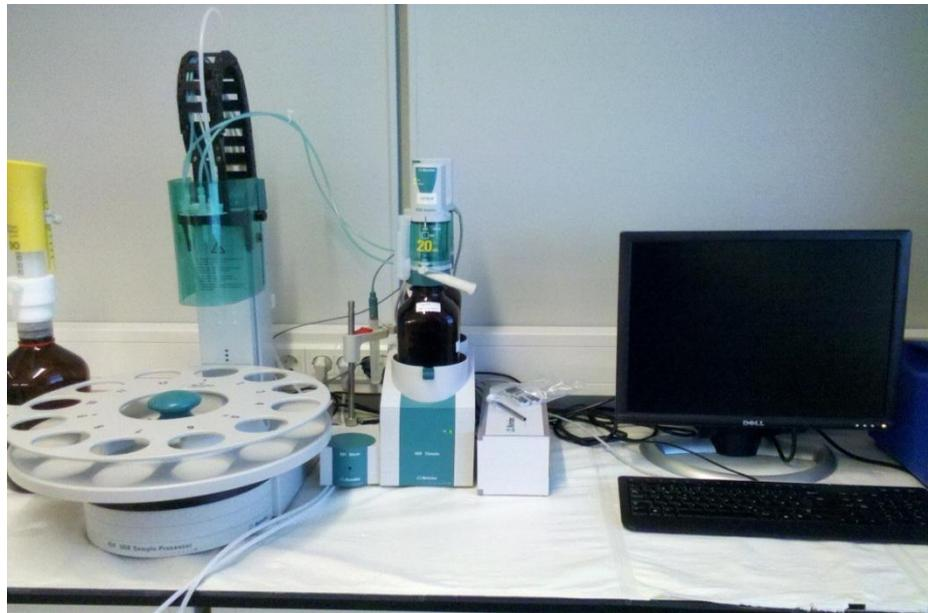
Figure 3.1(b) Metrohm 809 titrando setup for CO<sub>2</sub> analysis
