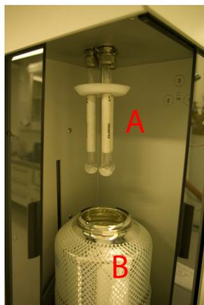
Figure 2.5: *Micromeritics TriStar 3000. A: Test tubes with samples. B: Raisable flask with liquid nitrogen.*
