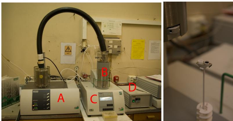
Figure 2.4: *Left: TGA/DTA set-up. A: Mass spectrometer. B: Furnace. C: Microbalance. D: Instrument and temperature controls. Right: Sample holder with sample and empty sample holder used as reference at top of the microbalance.*
