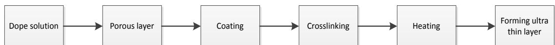
FIGURE 3.3(A) PROCESS DIAGRAM FOR SYNTHESIS OF COMPOSITE MEMBRANE (ADDAPTED FROM MULDER M., 1997)
