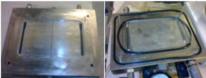
FIGURE 5.6 LIQUID AND GAS CHAMBERS OF MEMBRANE CELL
