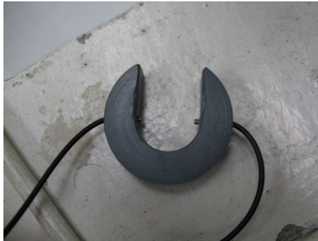
Figure 3.14: Fiber optic slug sensor by Omron.
