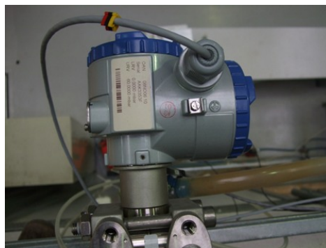
Figure 3.17: DP-Cell manufactured by Fuji with working pressure range of 0-6 kPa.
