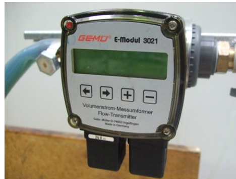
Figure 3.10: Liquid flow meter
