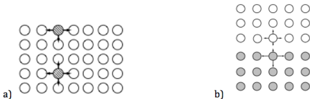
Figure 10: a) shows the origin of surface tension, while b) shows the origin of interfacial tension [36].
