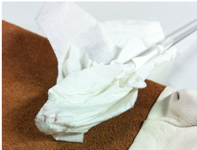
Figure 3-4 Deposits from steel fitting after cleaning with white tissue paper
