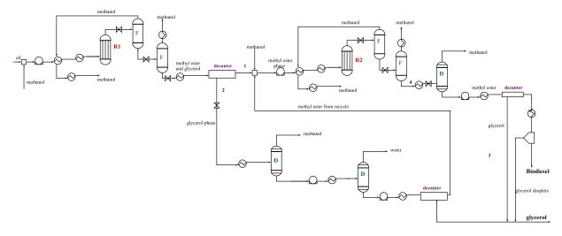
Figure B.1: Process flow sheet: The Esterfip-H process
