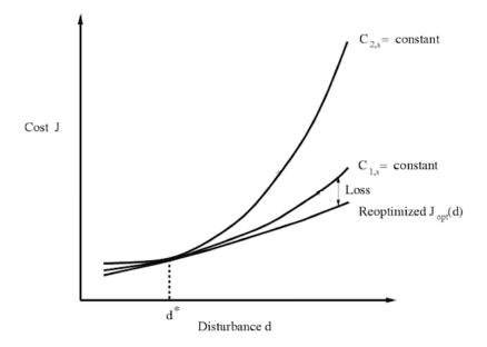
Figure 2.2: The different outcomes in terms of the cost function when the a process is reoptimized or controlled with self-optimizing control when a disturbance occur. [3]
