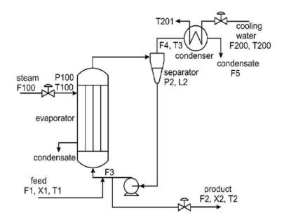
**Figure 5.1:** Flowsheet of the evaporator process as given in "Applied Process Control - A case study" by R.B Newell and P.L Lee [20],
