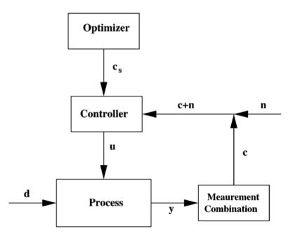
**Figure 2.1:** Dividing optimization and control into two layers can be illustrated in this way. Where the optimizer provides the set-points, and the controller tries to keep c=Hy at the constant set-point value when disturbances occur.[16]
