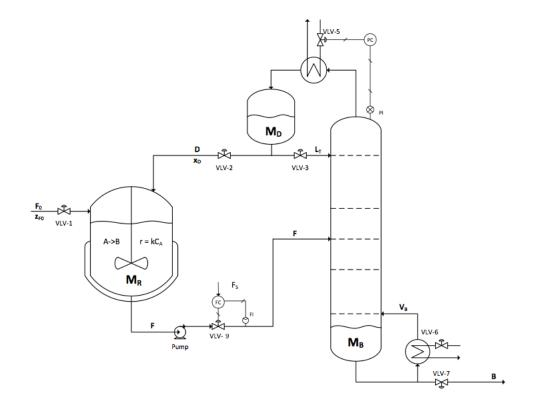
**Figure 6.1:** Process plant with a CSTR-reactor and a 22 stage distillation column with recycle [11].
