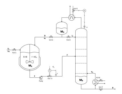
Figure A.1: Process plant with a CSTR-reactor and a 22 stage distillation column with recycle [11].
