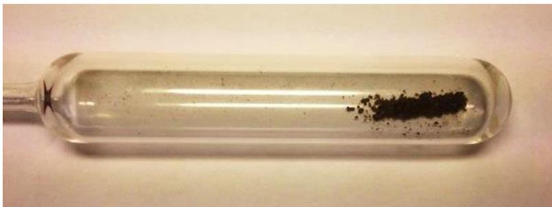
Figure 19 - Custom made glass tube with GO sample before thermal exfoliation [30].
