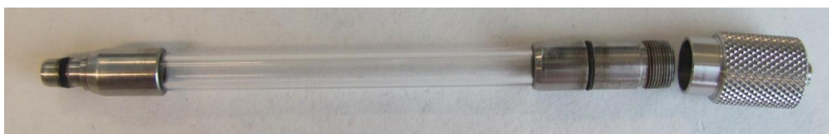
Figure 2.3: Capillary used for measurements in the spinning drop tensiometer.
