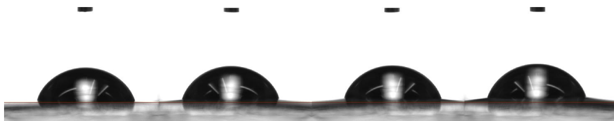
Figure 4-17: Water drop on membrane surface 1, 7, 11 and 30 seconds after drop impact. It can be seen how the membrane rises above the baseline. Pictures are placed side by side for easier comparison.
