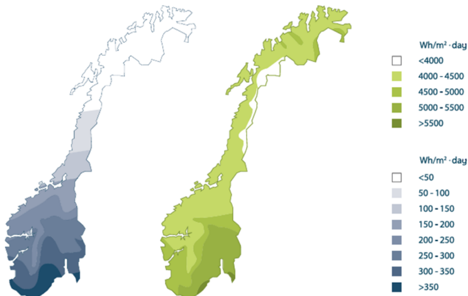
Figure 4.4: Daily solar irradiance incident on a horizontal plate in January and July respectively (SINTEF, 2007)
