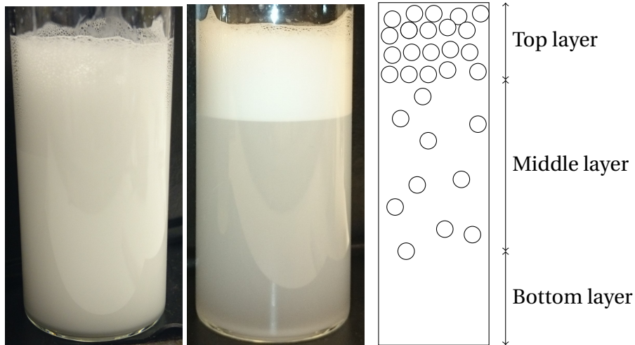
Figure 4.1: Oil-in-water emulsions immediately after preparation (left) and after layers have formed (middle). Illustration of the formation of emulsion layers (right).
