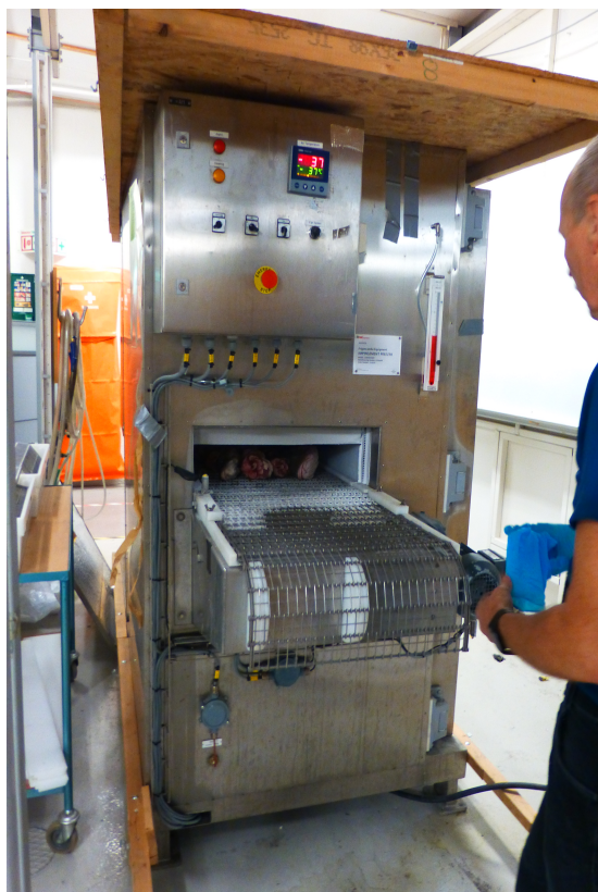
Figure 7. The impingement freezer used to freeze the raw material as the intact or vacuum-packed minced cod head at -37^{\circ}\text{C}
