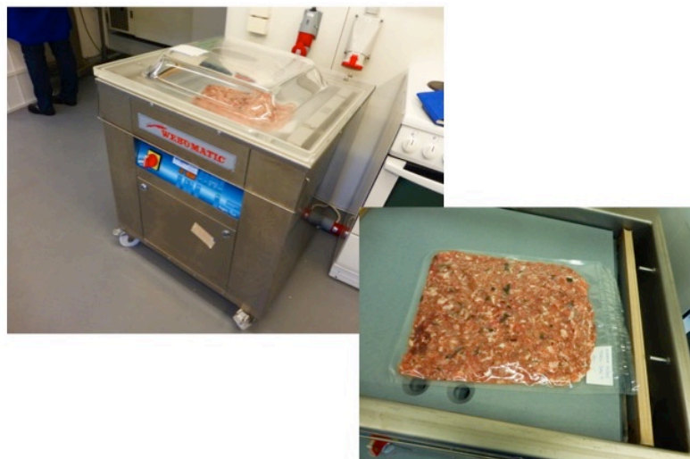
Figure 6. Minced cod head; the vacuum packing machine on the left and the vacuum-packed minced cod head on the right
