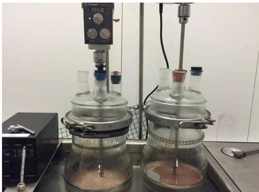
Figure 10. The reactor equipped with mechanical stirring placed in a water bath used for hydrolysis process of cod heads.
