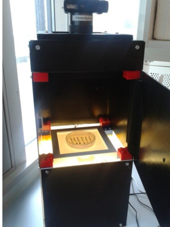
Figure 15 Custom-build stage. Plate with one of the iron or manganese sources placed on stage, where the digital camera is positioned vertically from the top.
