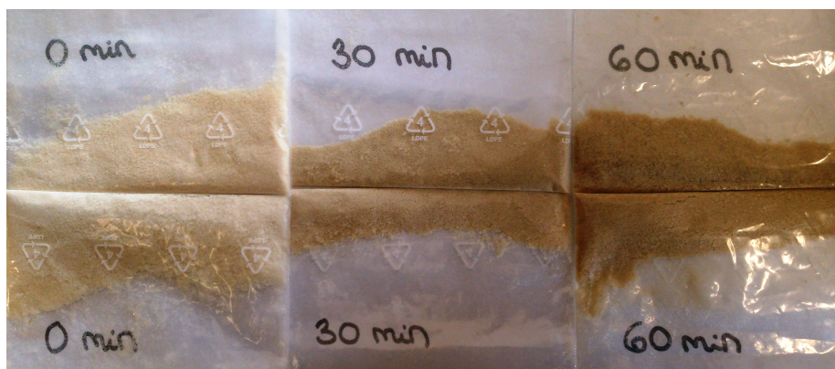
Figure 44: The colour of hydrolysates from reactor 2 after 0, 30 and 60 min of hydrolysis. The raw material was stored for 120 hours at either 10 °C (top) or 4 °C (bottom).
