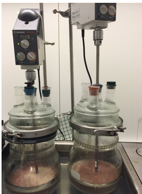
Figure 14: Experimental set-up for performing enzymatic hydrolysis. The 3 L closed batch reactor is placed in a water bath and the content is stirred using an electrical stirrer. The enzyme solution is added through the open tube in the lid and the lid is taken off for transferring rest raw material and water in and out of the reactor.
