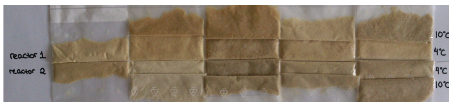
Figure 45: The colour of hydrolysates after 60 min of hydrolysis. From left to right: 0 h, 24 h, 48 h, 72 h and 120 h of storage of raw material. From top to bottom: reactor 1 - 10 °C, reactor 1 - 4 °C, reactor 2 - 4 °C and reactor 2 - 10 °C. Note that the hydrolysates furthest to the left in the picture (0 hours of storage) by a mistake have swapped places, the darkest sample belonging to reactor 1.
