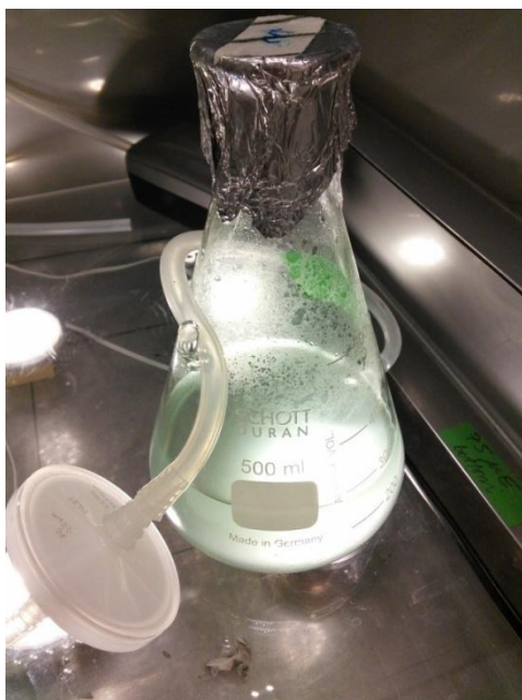
Figure 2.3 - 500 ml Erlenmeyer flask with 300 ml of BG11: Standard set-up for establishing a starter culture for PCC 6803.
