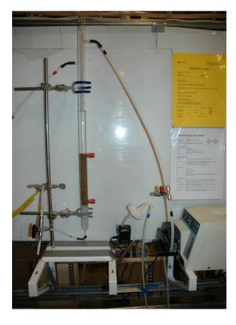
Figure 2.4: Bench-scale continuous flow biofilter.
