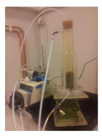
Figure 2.3: Batch biofilter column.
