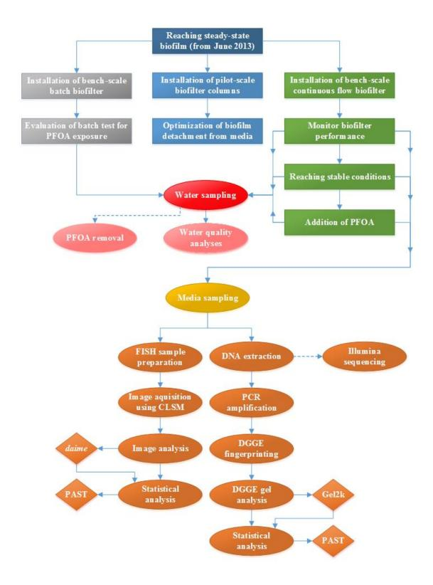
Figure 2.1: Experimental flow chart of activities, processes and experiments presented in this report. See text above the figure for more details about the flow scheme.
