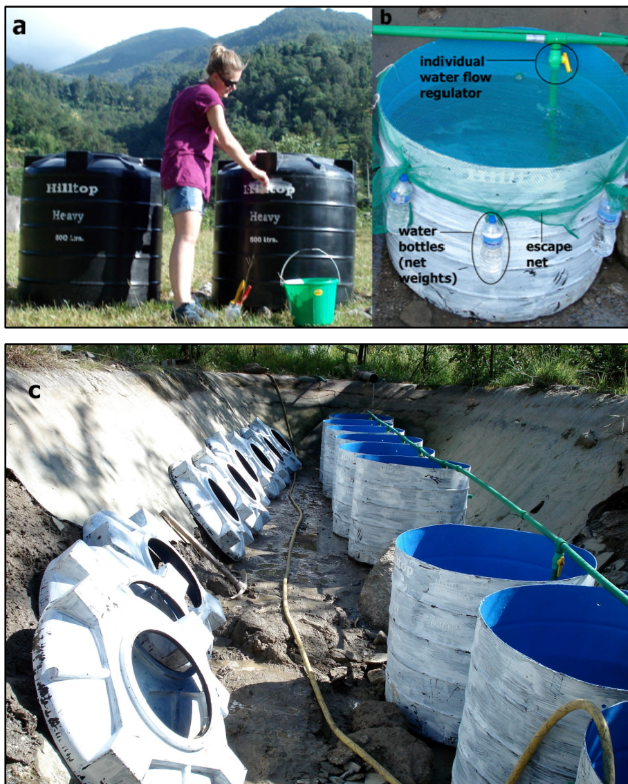
Figure 4: Adapting roof water tanks for fish experiment (a) The tanks before modification (b) modified tank for experimental use (c) the line of experimental tanks.
