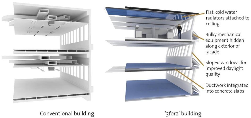
Figur 31: 3for2-konseptet (Laboratory, 2014)
